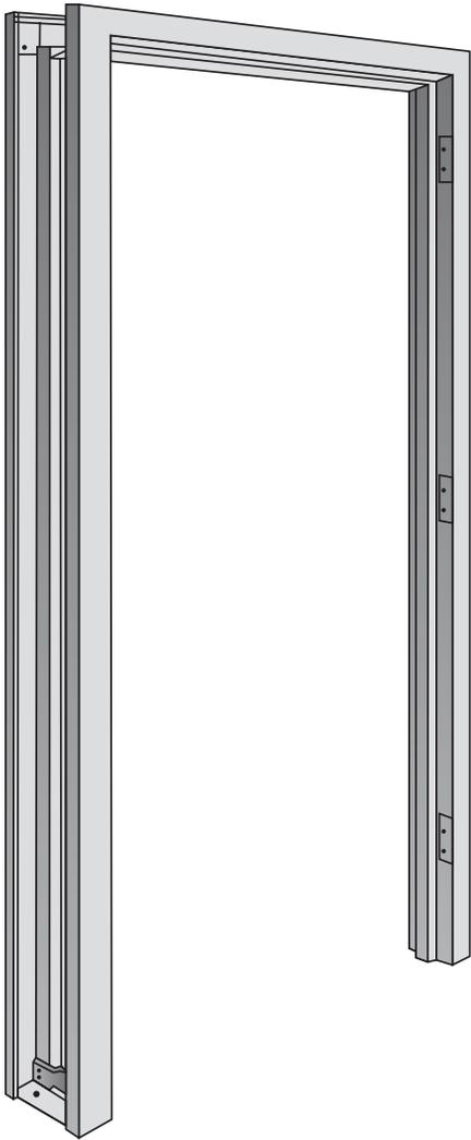
Our standard steel door frames are available in 14, 16 and 18 gauge wipe-coat galvanized steel and can be manufactured to meet all architectural design specifications. Warnock Hersey fire labeling is available when required. Standard profiles include 4-3/4", 5-3/4", 6-3/4" and 8-3/4".
