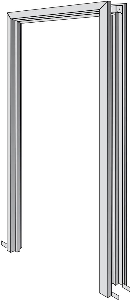
Our drywall frames are available in 18 gauge wipe-coat galvanized and 16 gauge. They can be accommodated any wall thickness and heavier interior applications. Standard drywall KDDW frames are available in 4-1/2", 5-5/8", 5-3/4" or 5-7/8" jamb depths.
