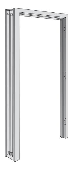
Our standard steel door frames are available in 14, 16 and 18 gauge wipe-coat galvanneal steel and can be manufactured to meet all architectural design specifications. Warnock Hersey fire labeling is available when required. Standard profiles include 4-3/4", 5-3/4", 6-3/4" and 8-3/4".
